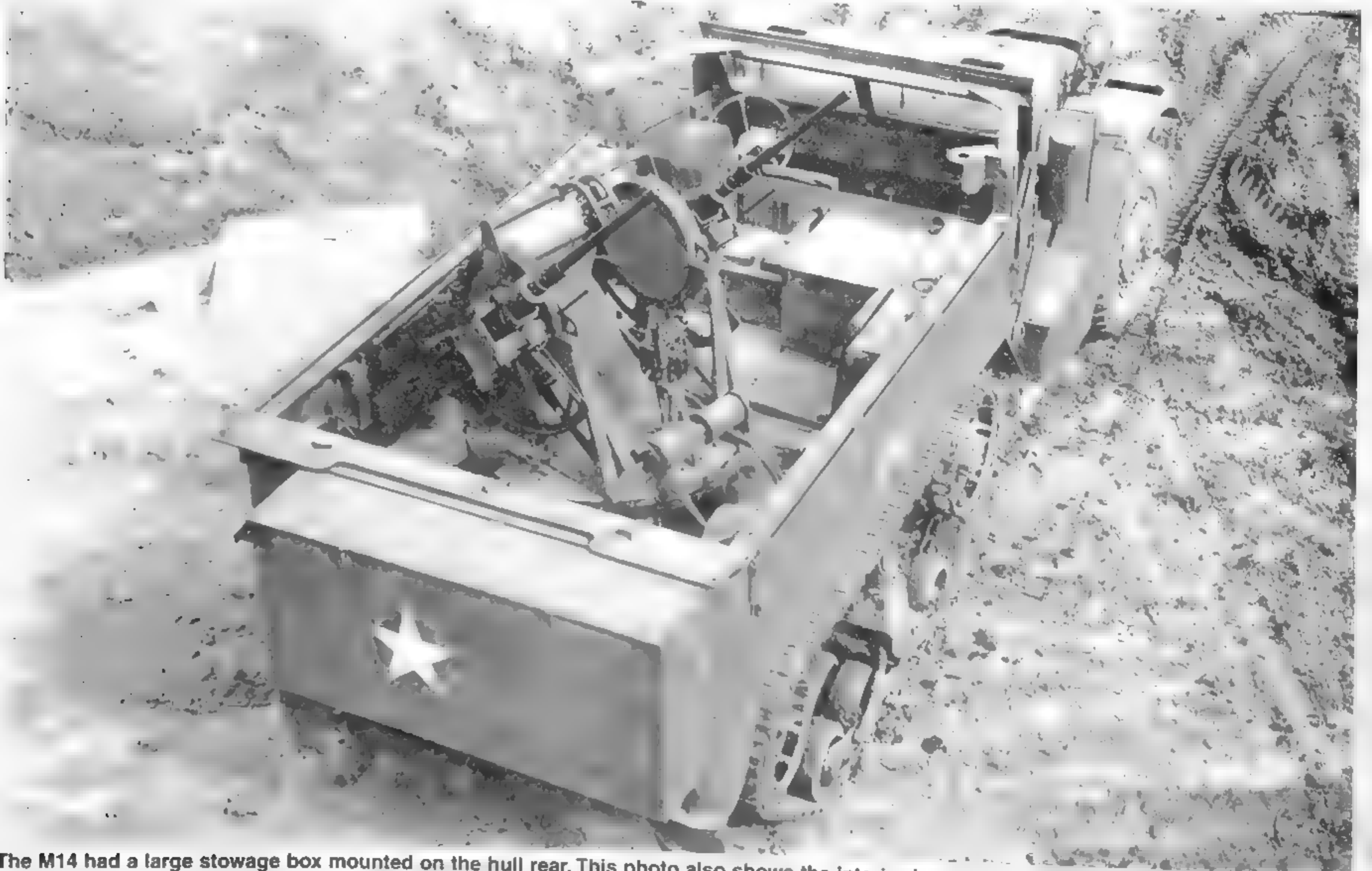
The folding side armor of the M14 Multiple Gun Motor Carriage is shown in this photo. This was necessary to provide a broad field of fire for the twin .50-caliber machine guns mounted in the M33 turret. (Photo courtesy of the Patton Museum)
